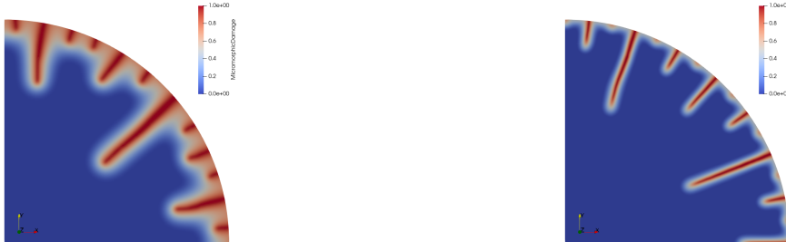
Figure 1: Microdamage at t = 0.950\text{s} for AT1, l_c/h = 6.74 Figure 2: Microdamage at t = 0.950\text{s} for Lorentz, l_c/h = 5.6
