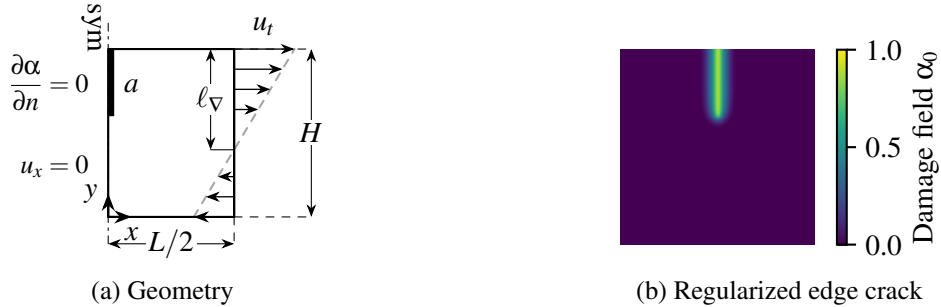
FIGURE 1 – Edge crack in a finite plate under non-uniform tensile loading inducing a stress gradient (on the left) and initial damage field \alpha_0 (on the right). The parameter \ell_\nabla controls the extent of the tensile region. Arrows indicate the direction of loading. The initial damage field \alpha_0 regularizes the edge crack of length a \approx 0.35H for zero loading t = 0 and \ell_{\text{PF}} = 0.05H .
